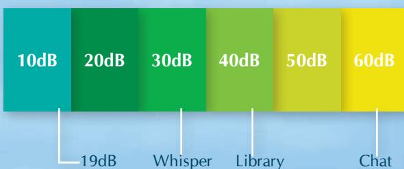
Noise level for silent mode operation is only at 19dB for MSY-GP10VF and MSXY-FP10,13VG making them one of the quiet units in the market. The multi-angled heat exchanger has a modified fin shape that reduces air resistance for a smoother, quieter airflow. The wide fan diameter produces great airflow at lower fan speeds and the uneven pitch between each fan blade helps to eliminate noise.
