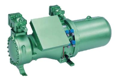
According to the actual operation condition, the system model can be adjusted by dedicated Microprocessor. And the slide valve fulfills the stepless control to enhance the efficiency under part load condition.
